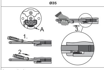
Insert a suitable flathead screwdriver between the locating lug and the snap-in pin, so that the snap-in pin releases the locating lug from the plug.
